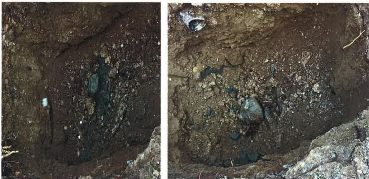
Photos 1 & 2 - Test pit #1 - Showing compacted clay mixed with gravel
