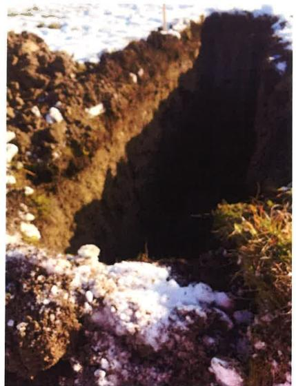
Photo #7- The Soil Strata below the topsoil - The Fill with light brown coloration.
