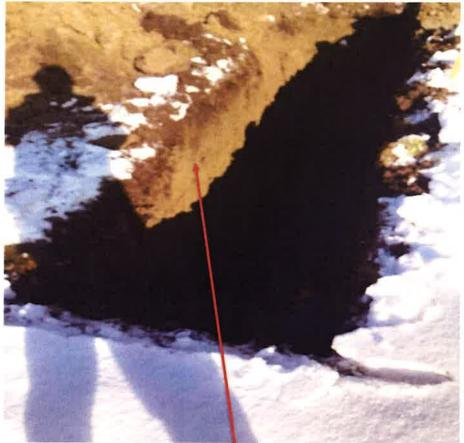
Photo # 5 - Test pit #1- silty clay
