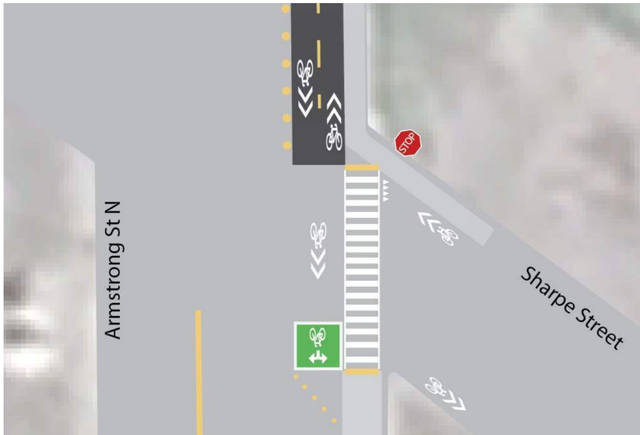
Figure 38 | Proposed left turn intervention at the intersection south of the bridge. (Yellow dots represent bollards, preferably mounted on pre-cast concrete curbs)
