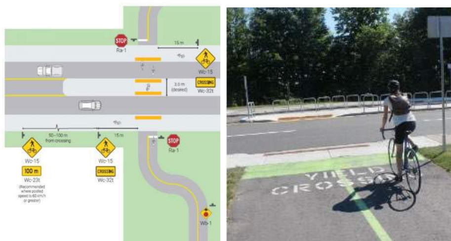
Figure 16 | Diagram illustrating the design elements of an uncontrolled mid block crossing and a photo of a sample application [Source OTM Book 18]
