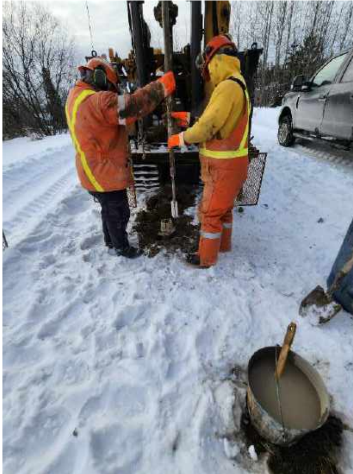
Photo 3- Crew of Landcore Drilling installing and preparing a Vane Shear
