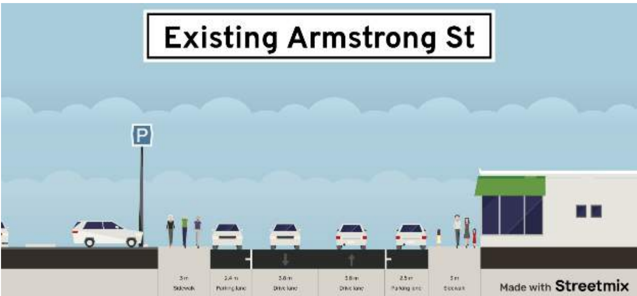
Figure 6-6: Typical Cross-Section – Armstrong Street
