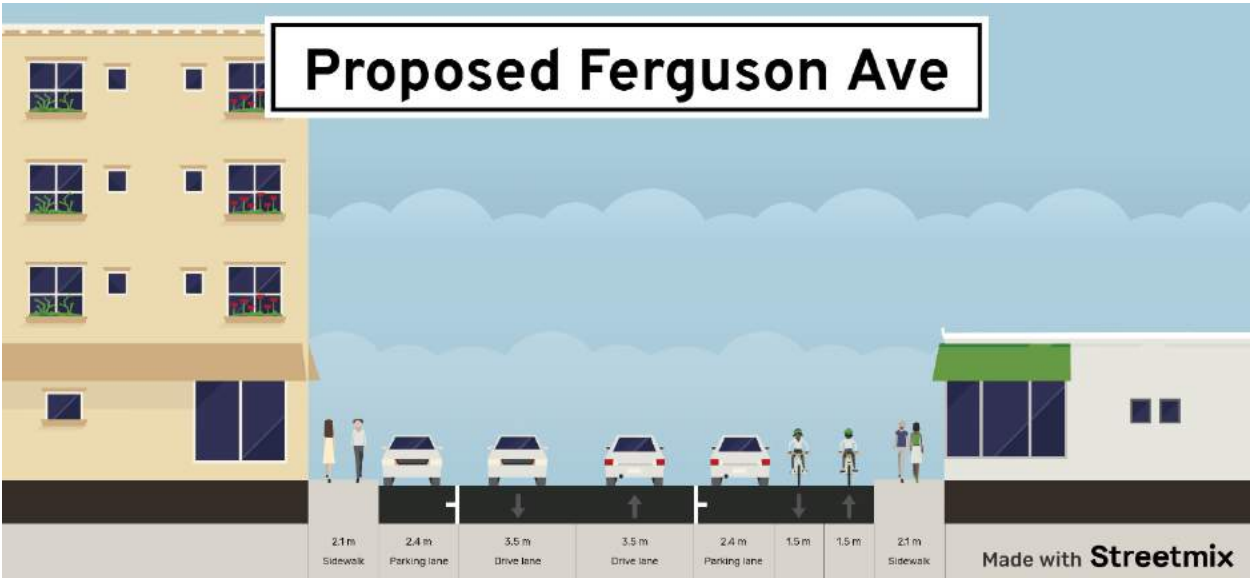
Figure 7-20: Proposed cross-section for Ferguson Avenue
