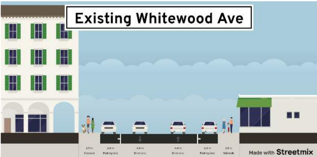
Figure 6-5: Typical Cross-Section – Whitewood Avenue
