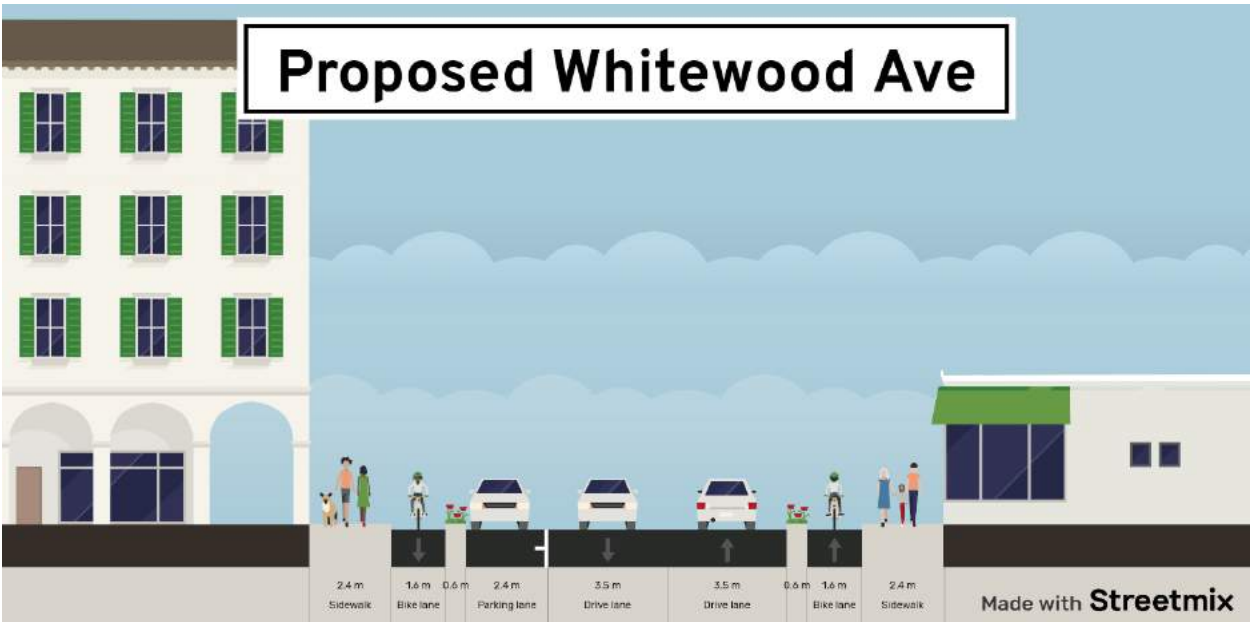
Figure 7-18: Proposed cross-section for Whitewood Avenue
