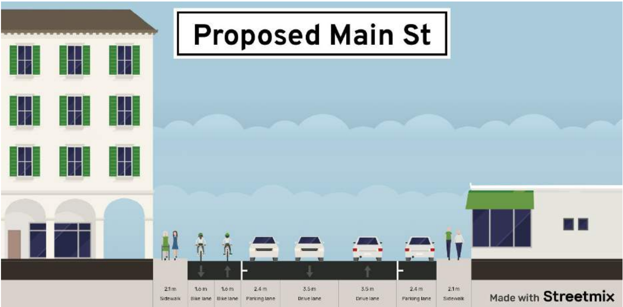
Figure 7-19: Proposed cross-section for Main Street
