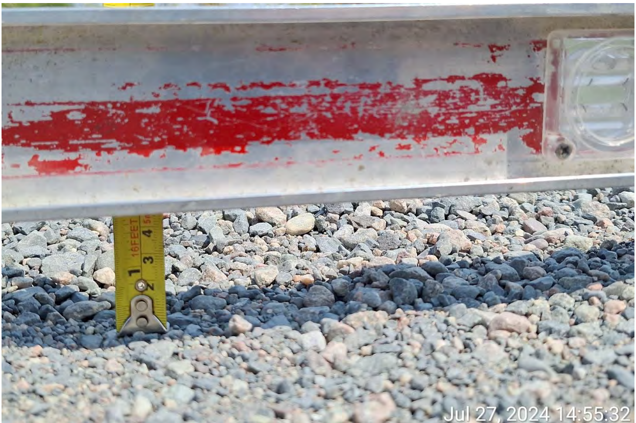
Figure 5: Washboard approximately 4.5cm deep
