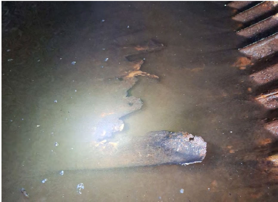
Figure 4 – Severely corroded bottom resulting in a piece being torn from the barrel
