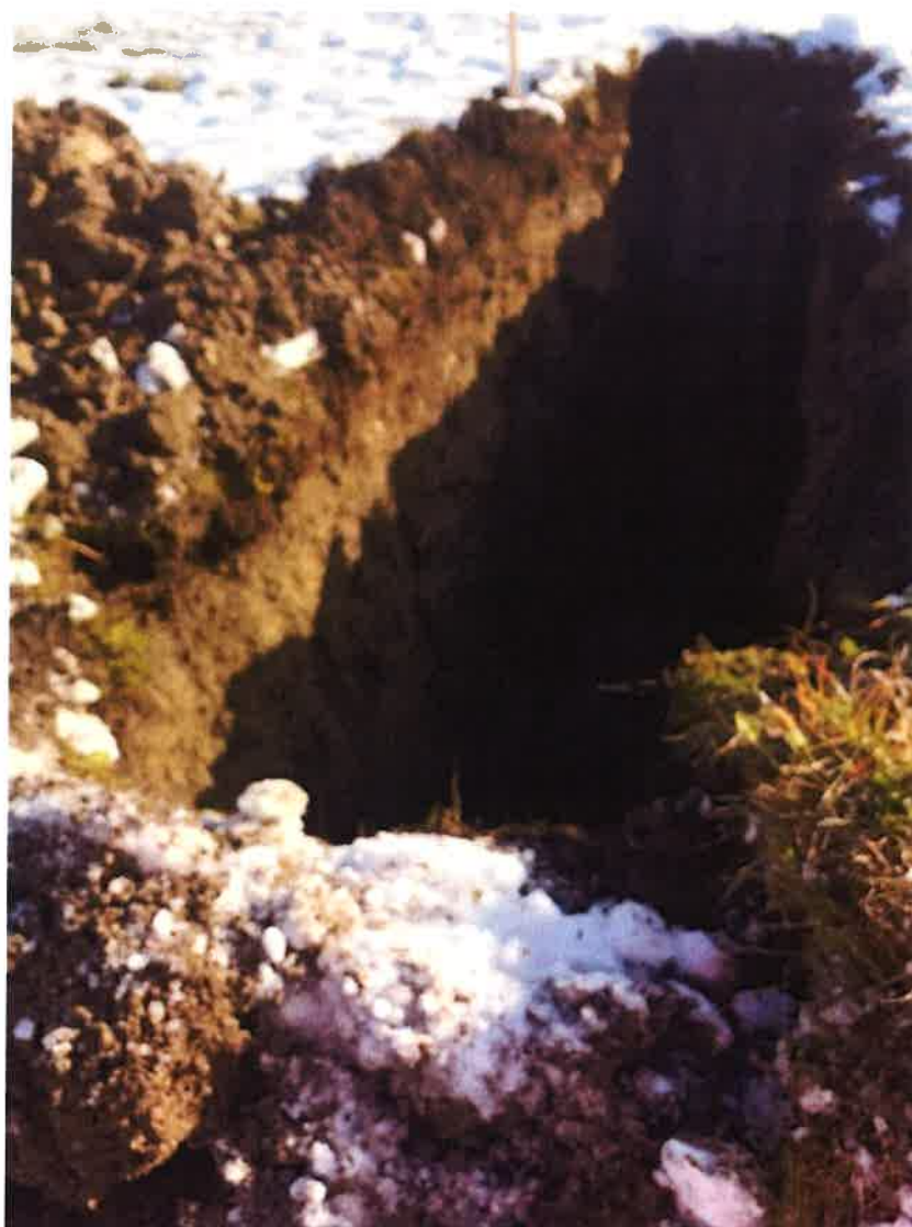
Photo #7- The Soil Strata below the topsoil – The Fill with light brown coloration.
