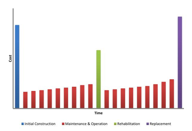
Figure 6.1: Accumulation of Costs Over an Asset's Life
