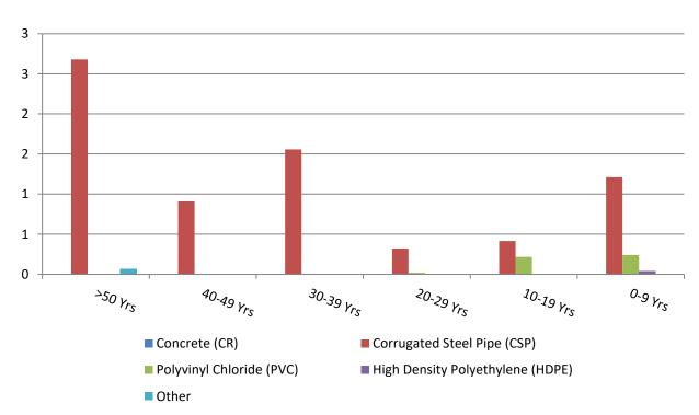
Figure 4.32: Length of Centerline Culvert Infrastructure Material by Age (Km)
