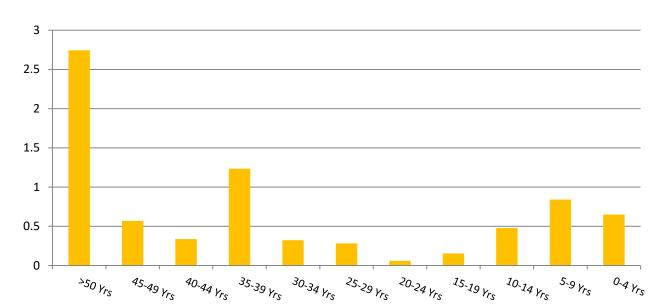
Figure 4.31: Length of Centerline Culvert Infrastructure by Age (Km)
