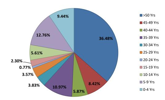
Figure 4.30: Centerline Culvert Infrastructure by Age (%)
