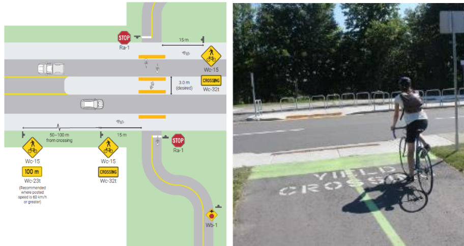
Figure 16 | Diagram illustrating the design elements of an uncontrolled mid block crossing and a photo of a sample application [Source OTM Book 18]
