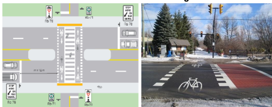
Figure 15 | Diagram illustrating the design elements of a signalized mid block crossing and a photo of a sample application [Source OTM Book 18]
