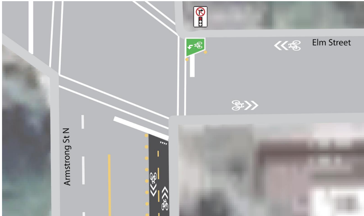
Figure 39 | Proposed left turn intervention at the intersection north of the bridge
