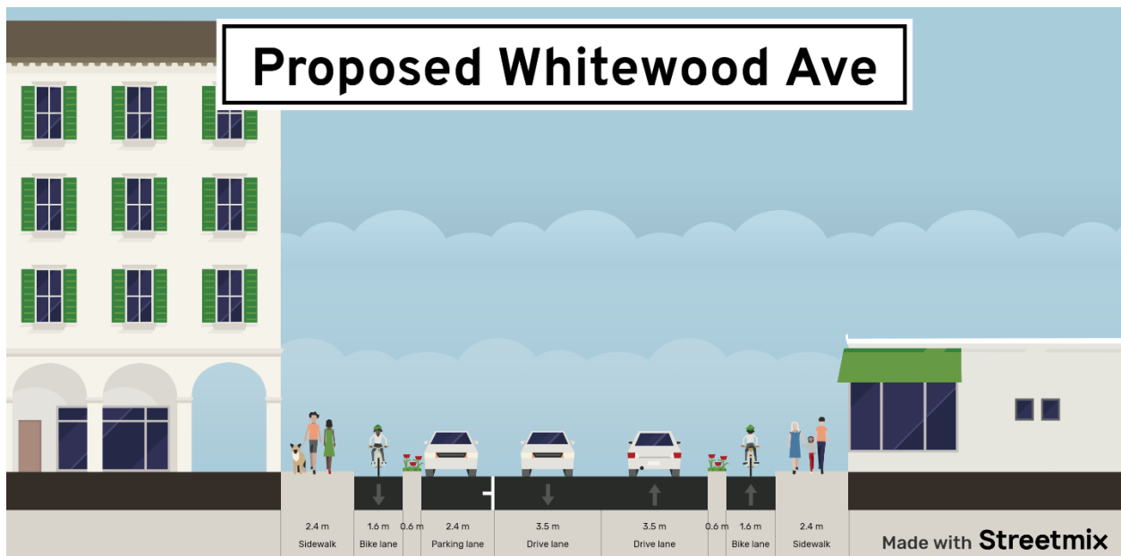
Figure 7-18: Proposed cross-section for Whitewood Avenue
