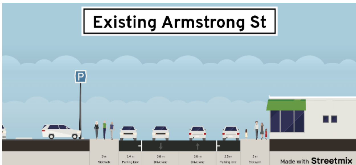
Figure 6-6: Typical Cross-Section – Armstrong Street
