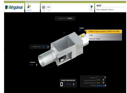
Figure 44: VVT1.3 - unable to obtain control point info
