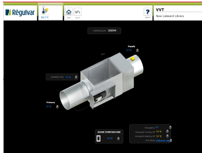
Figure 46: VVT1.4 - unable to obtain control point info
