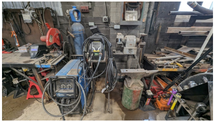
Figure 129: A - Chop saw, mig welder, plasma cutter, and grind wheel
