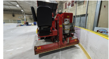
Figure 135: Manual ice leveller and propane fuelled ice resurfacer
