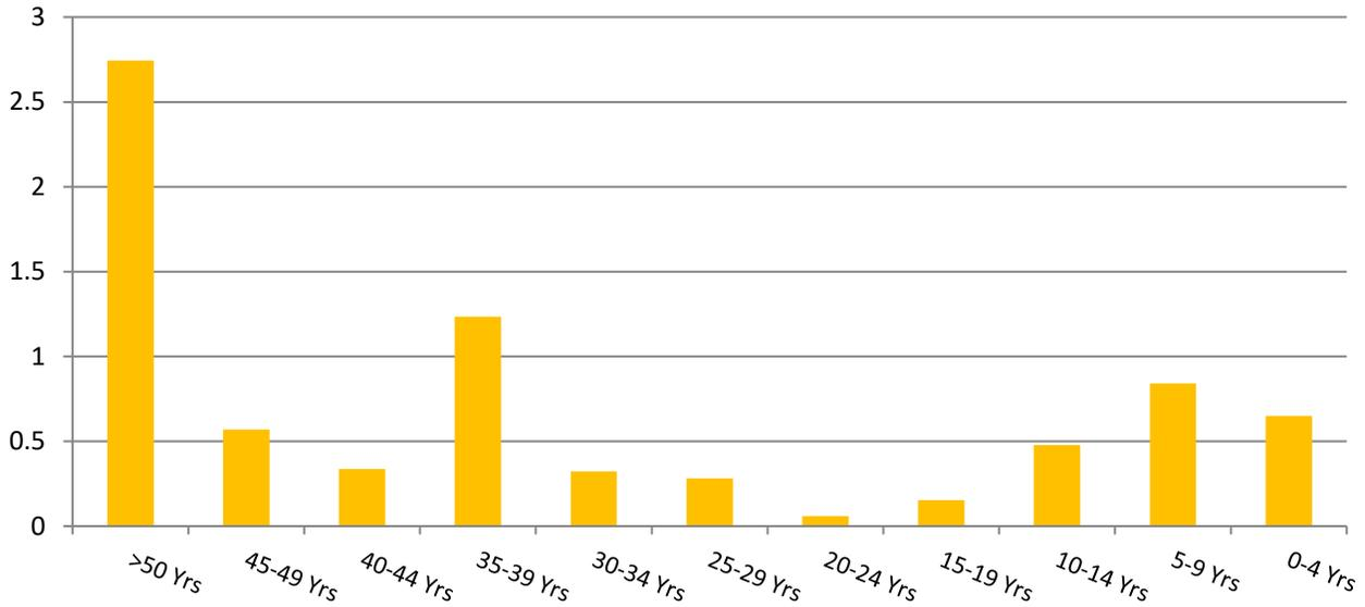
The majority of the culverts are Corrugated Steel Pipe with a diameter of over 1000 mm and installed over 50+ years ago, as shown in Figure 4.32, 4.33 and 4.34.
