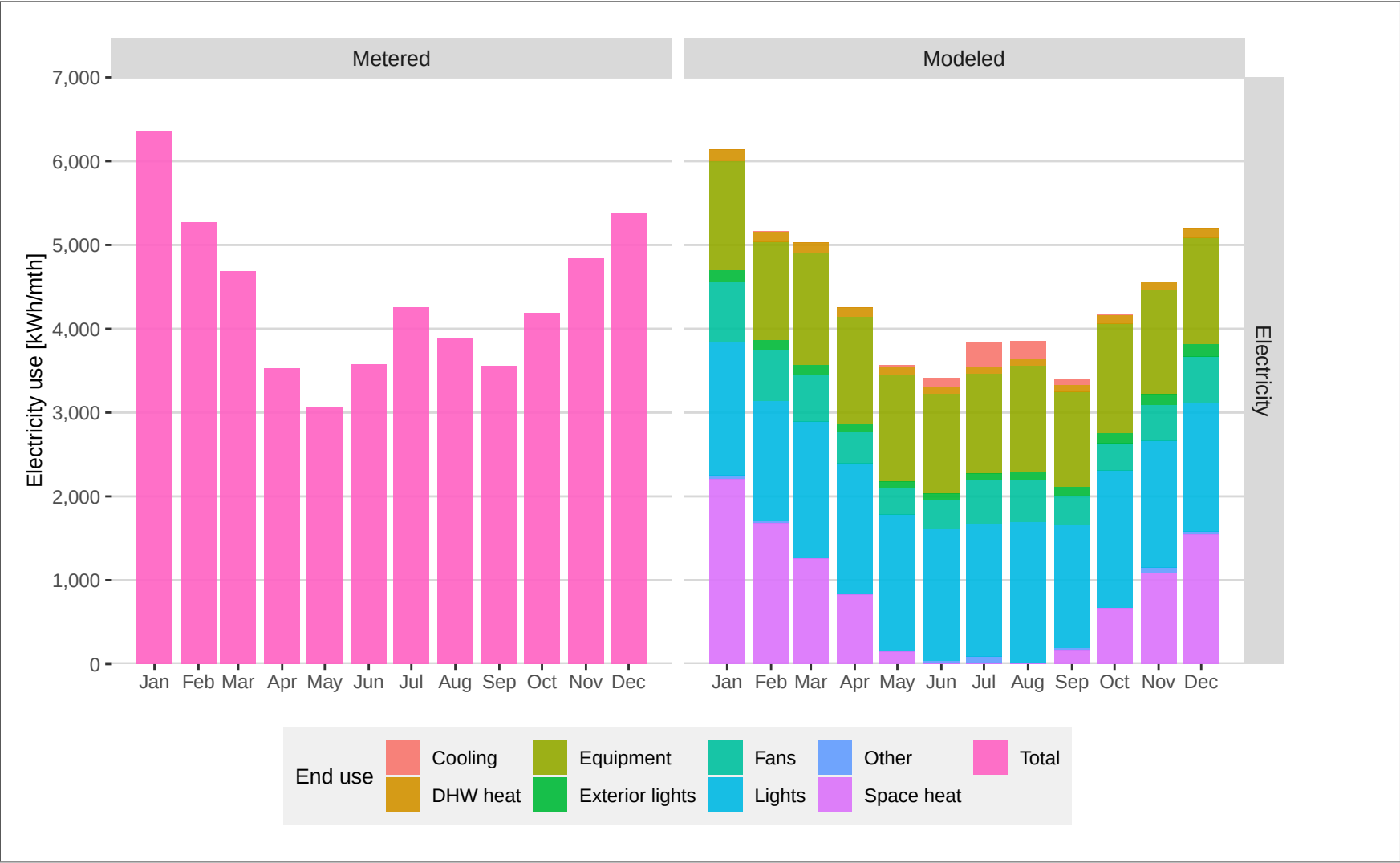
Figure 119: Electricity calibration analysis (metered vs modelled utility use)
