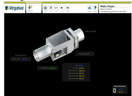
Figure 87: VAV - Main Foyer
