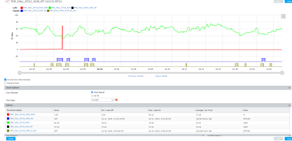
Figure 67: RTU2 - Humidity trend
