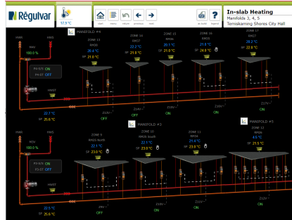
Figure 50: In-slab heating - Manifold 3, 4, and 5
